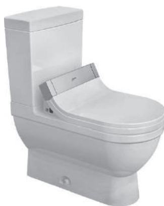
S/trap 305mm toilet 212551 / 610001 2-piece, with sensowash seat, conceal fixing
